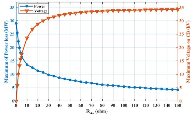
**Figure 18.** Maximum power loss and maximum voltage on switch ( $S_2$ ) based on resistor size ( $R_{dc}$ ) during start-up
