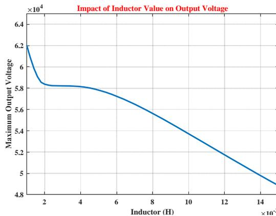
**Figure 5.** Overvoltage at start-up moment based on inductor value ( $C = 400\mu\text{F}$ )
