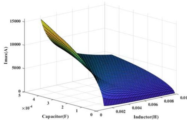
**Figure 9.** Simultaneous effect of change in capacitor and inductor values on start-up inrush current
