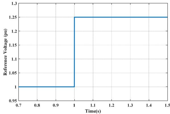
Figure 20. Conventional function for reference voltage signal
