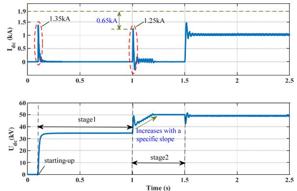
Figure 24. Simulation results of VSC-HVDC system with proposed control method
