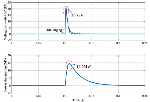
Figure 23. Power dissipation and blocking voltage S2 during starting-up process
