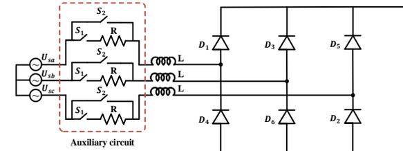
Figure 13. Starting-up diagram with three resistors and three CBs
