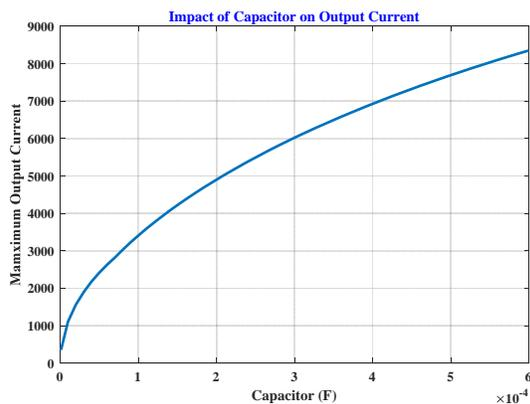
**Figure 6.** Inrush current at start-up moment based on capacitor value ( $L = 4.8\text{mH}$ )
