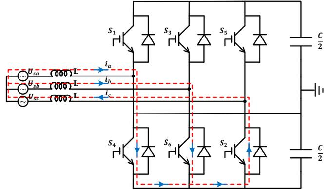
Figure 11. Lower switches are given a pulse and current flow in inductors from IGBT4, IGBT6 and D2 ( $i_a > 0, i_b > 0$  and  $i_c < 0$ )
