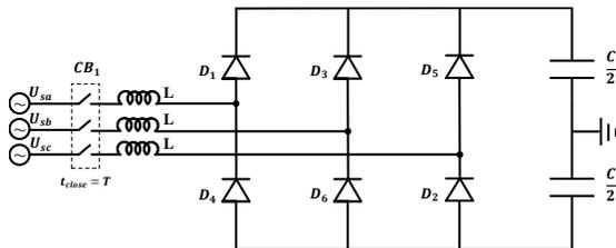
**Figure 2.** Equivalent circuit of uncontrolled rectifier stage without auxiliary starting-up system
