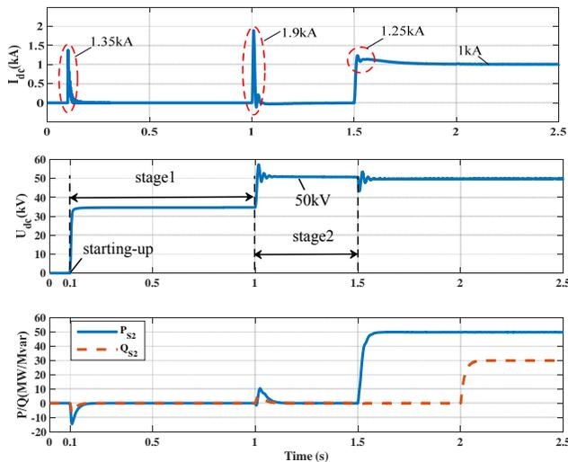
Figure 22. Simulation results of VSC-HVDC system with auxiliary starting-up system at DC side
