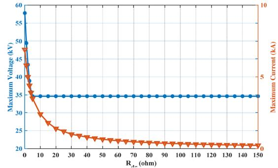
**Figure 17.** Maximum voltage and current curves based on resistor size ( $R_{dc}$ ) during start-up
