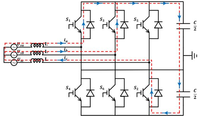
Figure 12. Current of the inductor pass through the capacitor from D1, D3 and D2 (Charging path)
