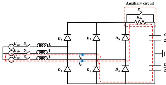
**Figure 16.** Starting-up diagram with one resistor and one switch at DC side
