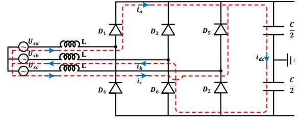
**Figure 3.** Currents path and charging capacitor path at the initial moment
