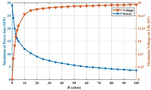
**Figure 15.** Maximum of power loss and voltage on the CBs ( $S_2$ ) based on resistor (R) during start-up
