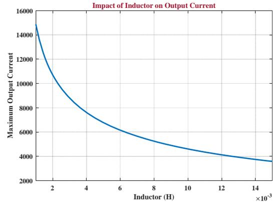
**Figure 7.** Inrush current at start-up moment based on inductor value ( $C = 400\mu\text{F}$ )
