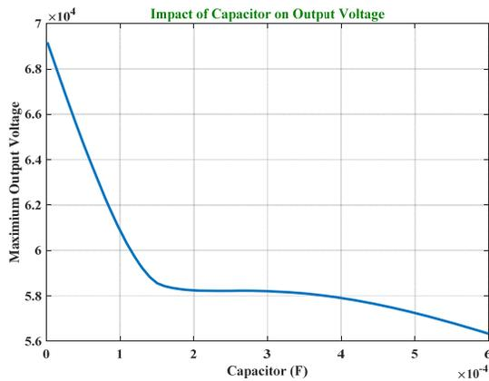
**Figure 4.** Overvoltage at start-up moment based on capacitor value ( $L = 4.8\text{mH}$ )
