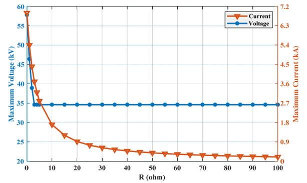
**Figure 14.** Maximum voltage and current based on resistor (R) during start-up
