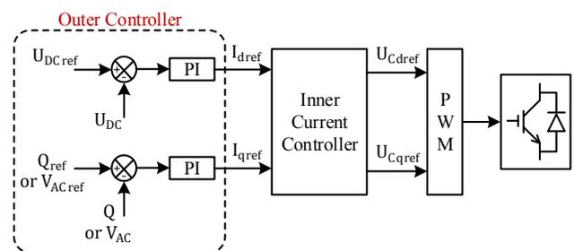
**Figure 19.** The control diagram of VSC-HVDC
