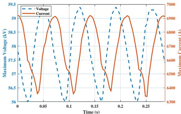
**Figure 10.** Impact of CBs closing time on overvoltage and inrush current ( $C = 400\mu F, L = 4.8mH$ )
