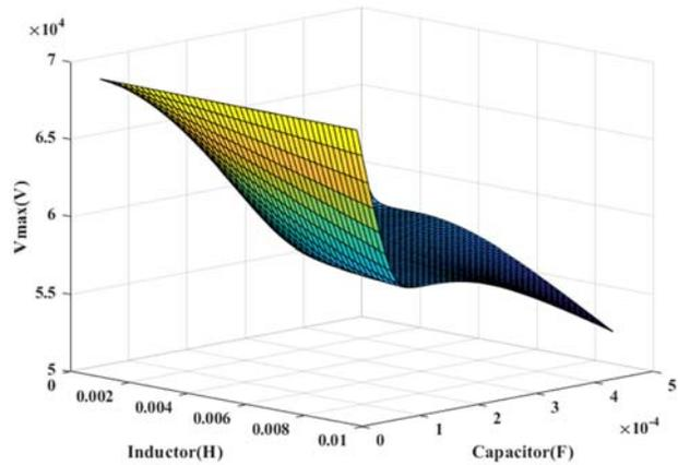
**Figure 8.** Simultaneous effect of change in capacitor and inductor values on start-up overvoltage
