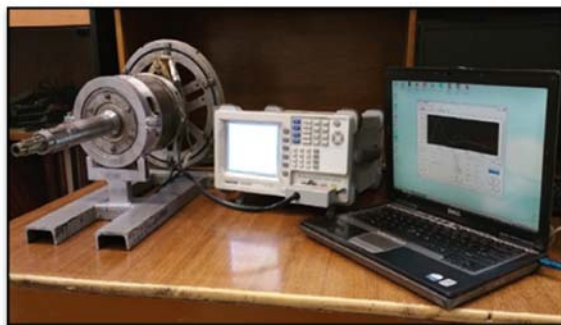
Fig. 4. Test 8kw PMSM impedance measurement setup
