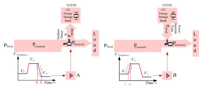
Figure. 6. UCES CONTROLLER, STORAGE /INJECTION OF ENERGY
