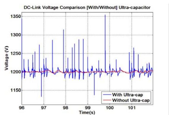
Fig. 16. MAGNIFIED DC-LINK VOLTAGE COMPARISON [WITH/WITHOUT] UCESB
