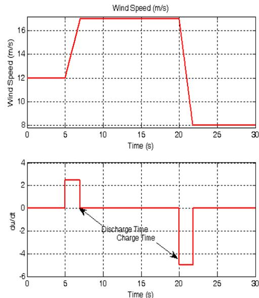
**Fig. 11. DETECTION OF WSVS FROM WIND SAMPLE**
