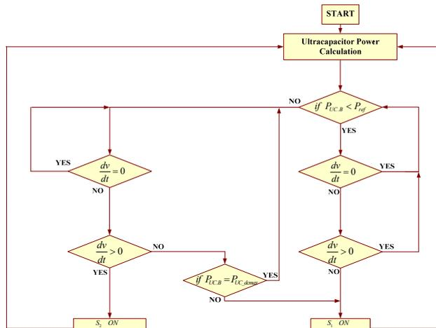
**Fig. 8. LITHIUM-ION UCES FLOWCHART (OBSERVATION & CONTROL) METHOD FOR POWER IMPROVEMENT**
