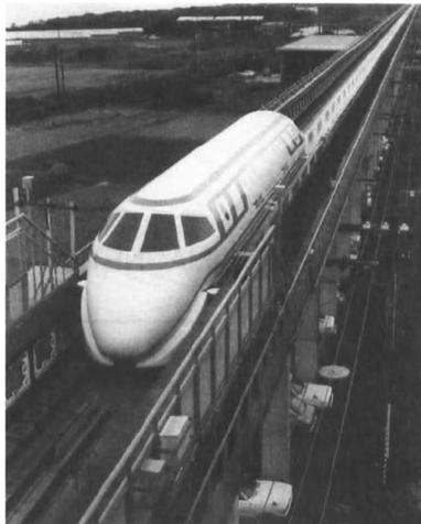
**Fig. 1.** PHOTOGRAPH OF JAPANESE SUPERCONDUCTING MAG-LEV VEHICLE; RATED SPEED 500 km/hr [4].
