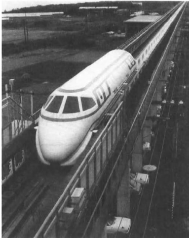
Fig. 1. PHOTOGRAPH OF JAPANESE SUPERCONDUCTING MAG-LEV VEHICLE; RATED SPEED 500 km/hr [4].
