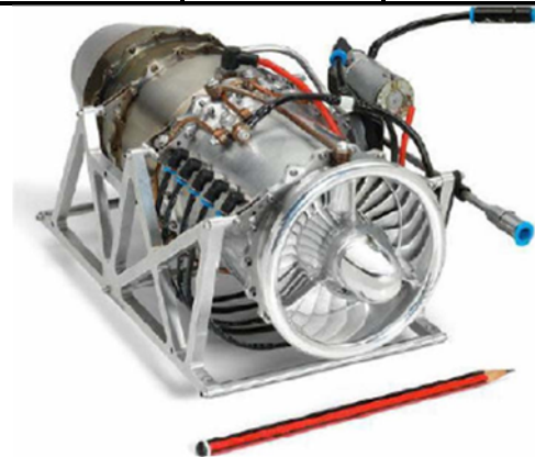
Fig. 7. Microturbine manufactured by Bladon Co.
