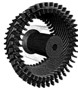
Fig. 29. End-region, rotor and stator winding and rotor shaft [34]
