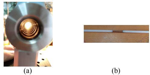
Fig. 12: Practical prototype of the inner stator resolver with five projections a) Slotted section b) Reluctance variation section
