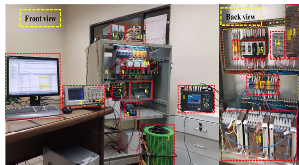
Fig. 15. Experimental setup; 1- Power Analyzer, 2- Auto transformer, 3- Code Composer Studio, 4- Scope, 5- Multi-meter, 6- Protection board, 7- Control board, 8- Digital to Analog Board, 9- Heat sink, 10- IGBT driver, 11- Capacitor bank, 12- Power supply 12VDC, 13- Power supply 12VDC, 14- Power supply 5VDC, 15- Relay contactors, 16- Pre-charge resistors, 17- Terminals, 18- Inductors
